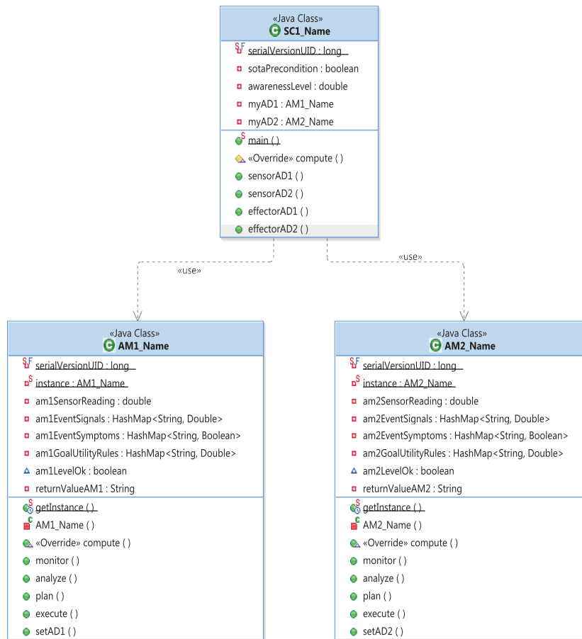
Figure 17: Java pattern template model of the parallel AMs SC pattern [AHZ15].
