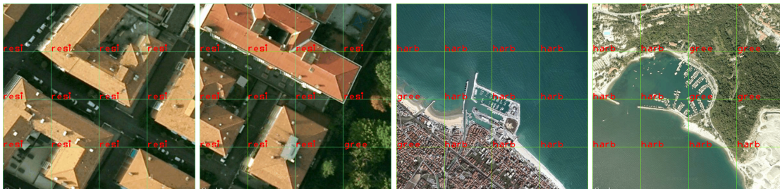
Figure 4: Four snapshots taken from the location sensor using satellite imagery. Residential and harbour areas are correctly classified. The red strings superimposed on map tiles are actual classification labels produced by the sensor. Table 4 summarizes the complete confusion matrix.
